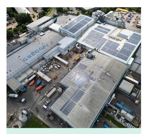
Project Greggs' Factory Value £220,000 At Greggs' factory in the northeast, we have begun installation of a 421.5 kWp system. The system will produce a predicted 361,463kWh in its initial 12 months of operation. This will save 83.5 tonnes of carbon in the systems initial year, or the equivalent to over 520 trees.
